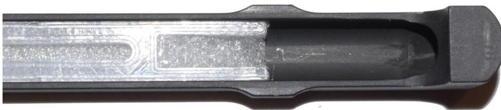
Proper positioning is shown in the above photo. Please note that placing the insert too far towards the front of the charging handle may result in interference with the rifle's gas tube, and may cause malfunctions and/or damage to the gas tube if forced closed.
