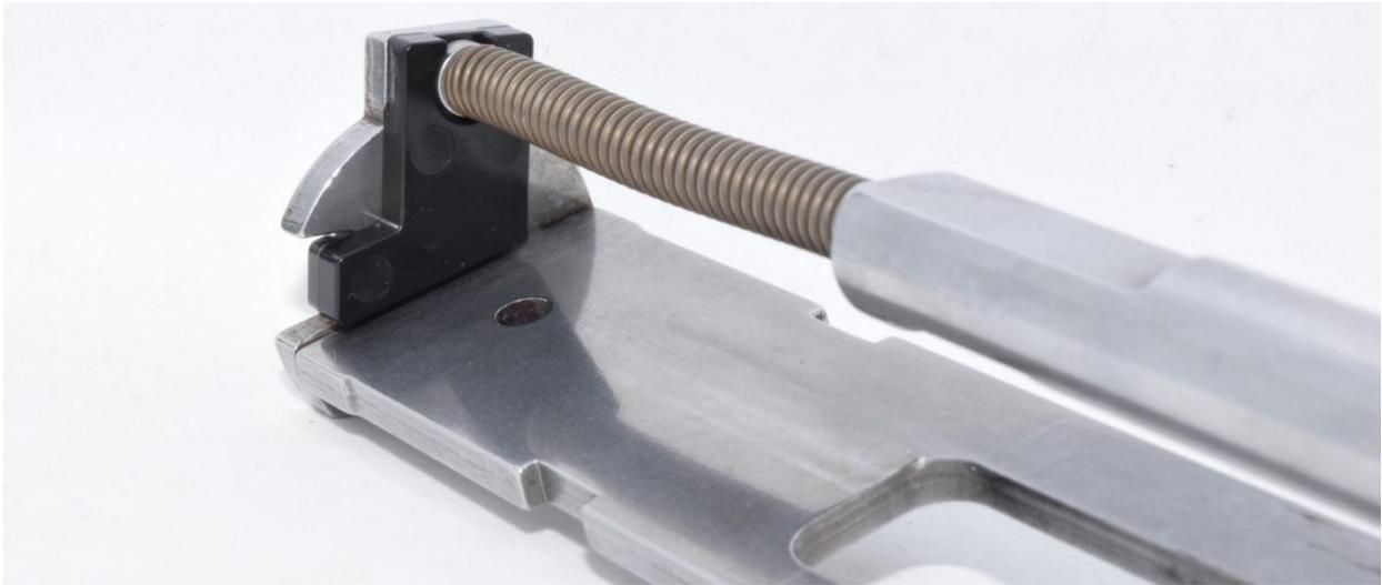
Note: if you have an older kit without the cutout on the back plate, the tab on the buffer can be clipped off. The buffer will not automatically align with the upper receiver without the tab, so care will be needed when replacing the bolt carrier assembly into the upper receiver to prevent binding from the buffer rotating.
